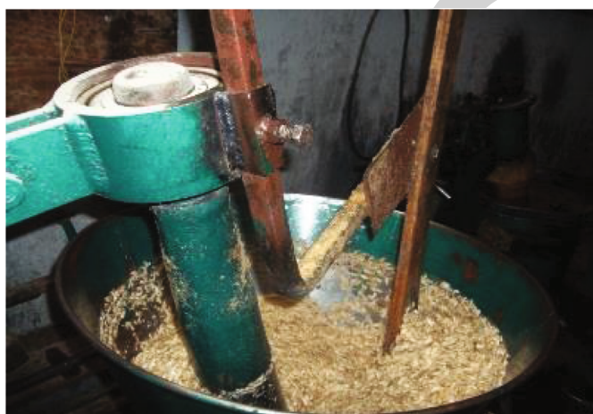
FIGURE 2: Oil extraction machine with sapodilla inner seed kernels.
