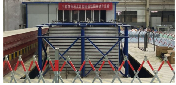
FIGURE 5: Shaking-table testing system.
