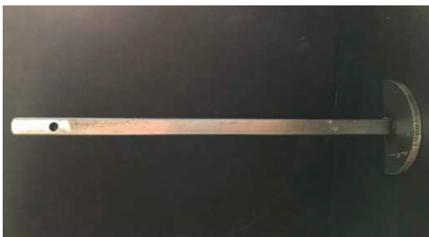
FIGURE 3: Plate anchor style.
