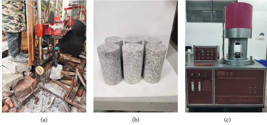
FIGURE 3: Production process and core samples of quartz diorite. (a) Core processing. (b) Rock samples. (c) Rock triaxial loading device.
