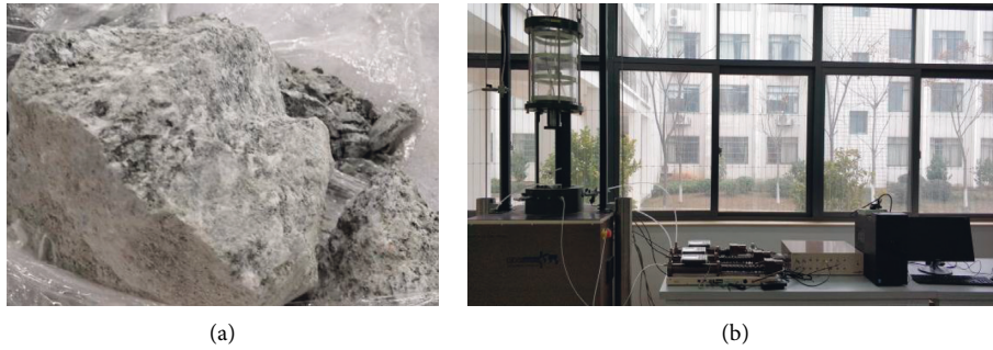
FIGURE 4: Strongly weathered quartz sandstone and test instruments. (a) Strongly weathered quartz sandstone. (b) GDS hollow cylinder torsional shear instrument.
