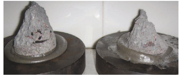
FIGURE 24: The failure of specimens under dynamic pressure.
