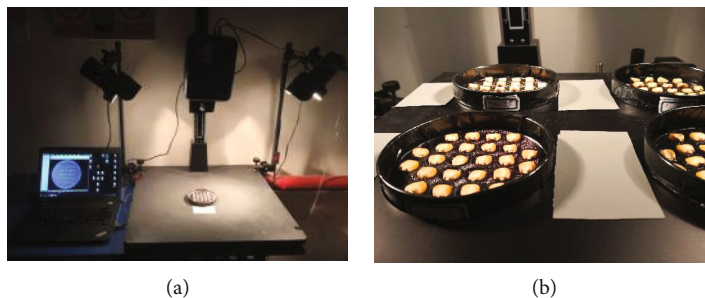
FIGURE 4: (a) Hyperspectral imaging system; (b) corn samples in Petri dishes.
