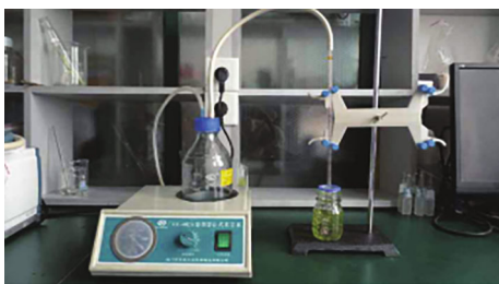
FIGURE 8: Breakthrough vacuum experimental device [44].
