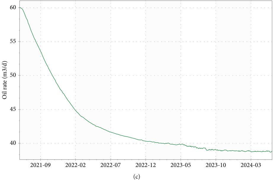
FIGURE 16: Sidetracking effect on the residual oil near the L19 well.
