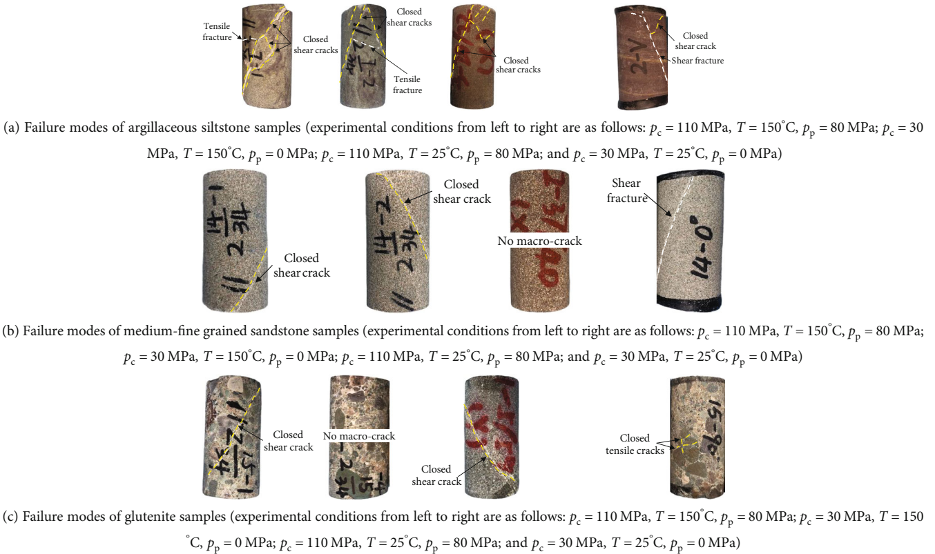
FIGURE 3: Illustrations of failure modes of samples with different lithologies under high temperature and high pressure.
