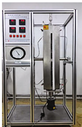
(a) YP-1 high-temperature, high-pressure gel performance test device
