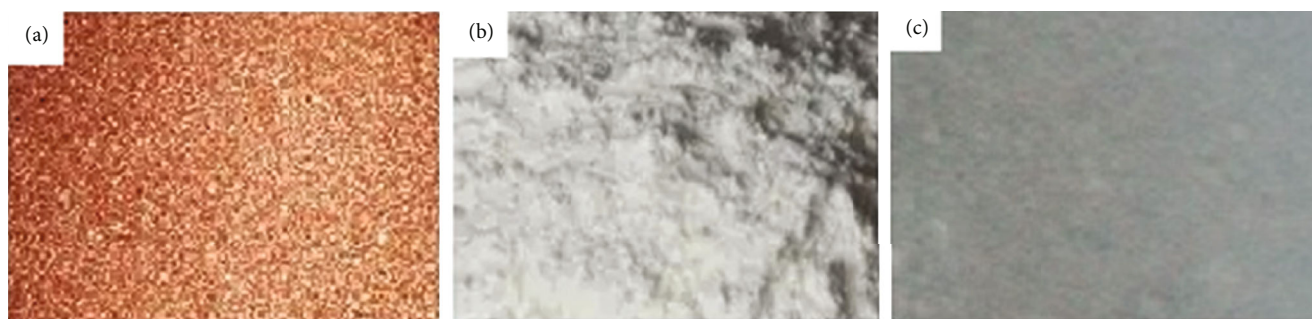
FIGURE 1: Actual illustrations for (a) copper metal particles, (b) alumina nanoparticles, and (c) graphite nanoparticles.
