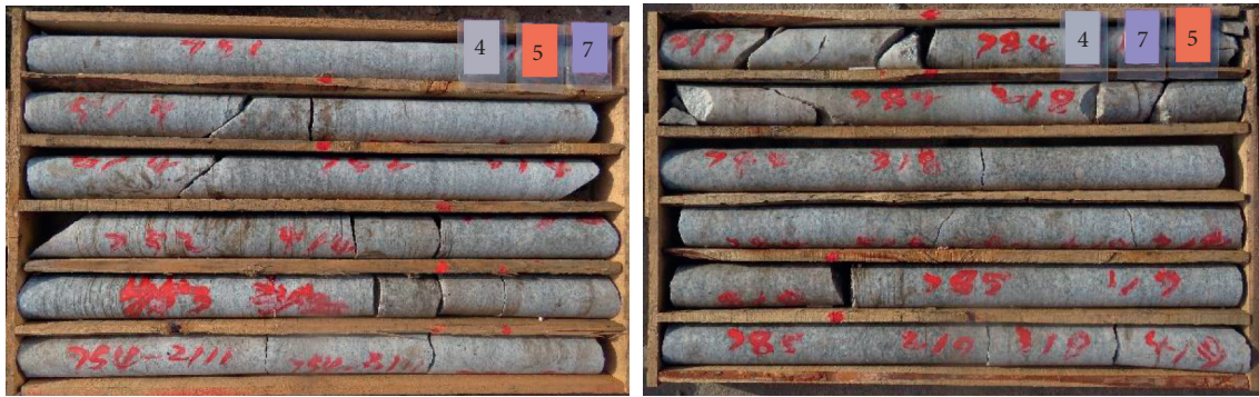
FIGURE 3: Core exposure of some strata (–1815.56~–1820.16 m, –1897.46~–1902.06 m).
