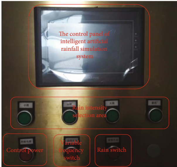
FIGURE 3: The rainfall control system.
