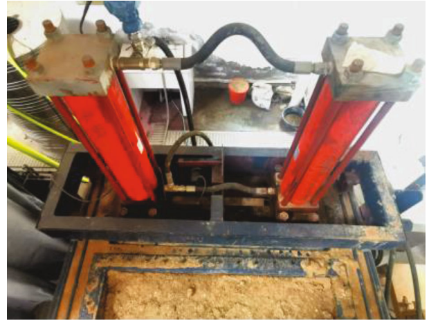
FIGURE 6: The ground stress loading system [42].
