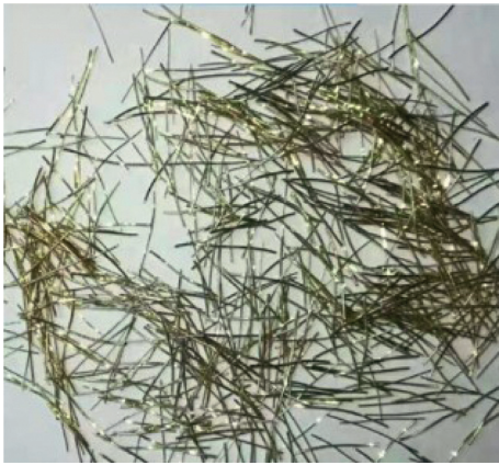
FIGURE 1: The shape of steel fibers.
