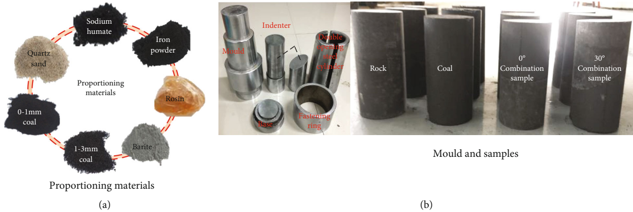
FIGURE 1: Sample preparation materials and standard samples: (a) proportioning materials, (b) mould, and samples.
