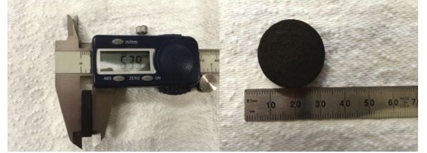
FIGURE 4: Photograph of a slice of the Marcellus shale drilled core sample cut into a disk with 5.39 mm in thickness and 25.4 mm in diameter.
