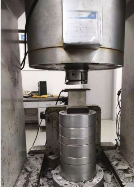
FIGURE 2: Compressive strength test of composite material specimen.
