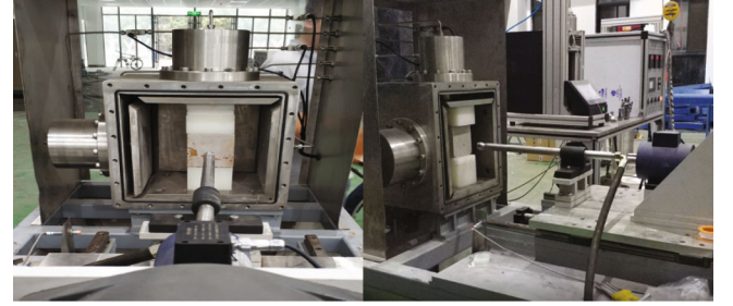
FIGURE 7: Physical diagram of a test block fixing device.
