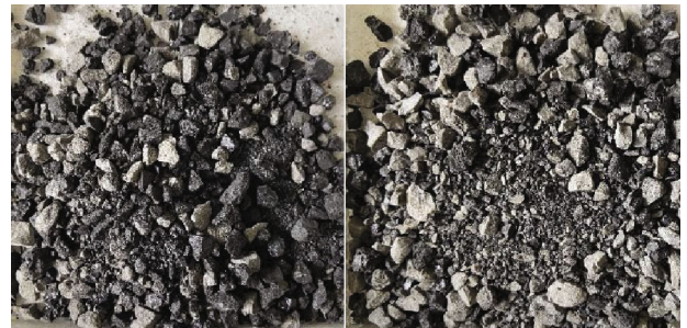
FIGURE 10: C2 and C3 samples after loading and unloading cycle.
