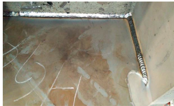
FIGURE 3: Design of steel box girder: (a) cross section of the steel box girder; (b) section diagram of the steel box girder; (c) bulb flat ribs welding; (d) diaphragm-bulb flat rib weld (unit: mm).
