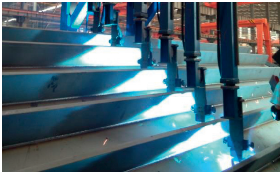
FIGURE 3: Design of steel box girder: (a) cross section of the steel box girder; (b) section diagram of the steel box girder; (c) bulb flat ribs welding; (d) diaphragm-bulb flat rib weld (unit: mm).
