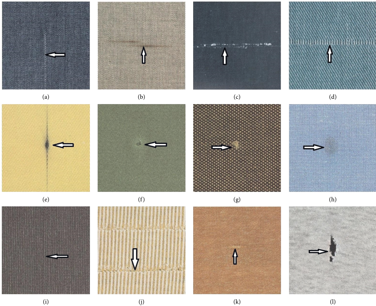
FIGURE 1: Some fabric defects which occur during manufacturing processing: (a) end-out, (b) soiled-filling, (c) sloughed-filling, (d) mispick, (e) soiled-end, (f) warp-slab, (g) knot, (h) oil spot, (i) end-out, (j) missing-yarn (k) slub (l) hole.
