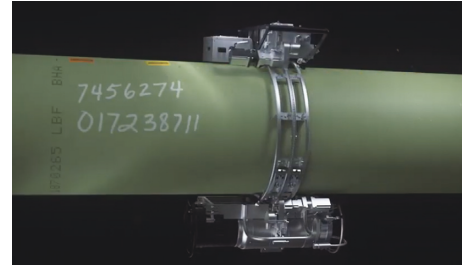
FIGURE 1: Digital X-ray detector and source on a robotic platform, Stanley Oil and Gas.
