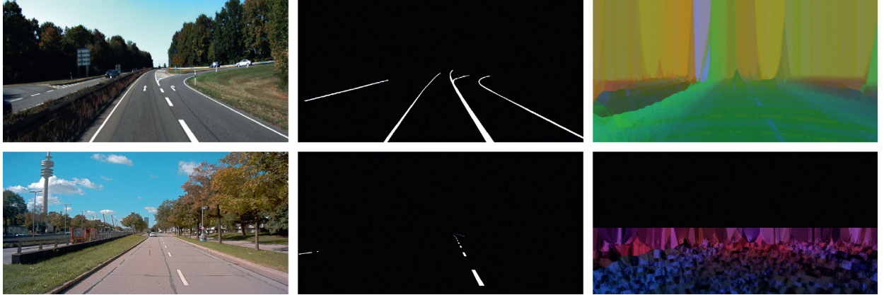
FIGURE 6: Examples of KITTI(top row) and A2D2(bottom row). The columns from left to right are camera image, lane line label, and point cloud.
