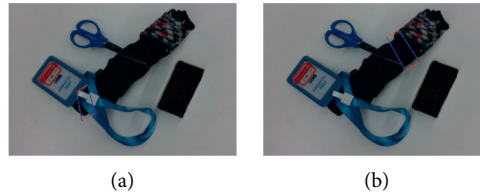
FIGURE 7: Comparison of our matching algorithm with the original SIFT algorithm on household objects: (a) the result generated by the original SIFT algorithm; (b) the result obtained by our matching algorithm. Our matching algorithm decreases the influence of occluded parts and predicts a more suitable grasp configuration than the original SIFT algorithm.
