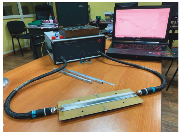
FIGURE 4: Vector network analyzer «Panorama» P4226 and an MF prototype with a corner passive conductor.
