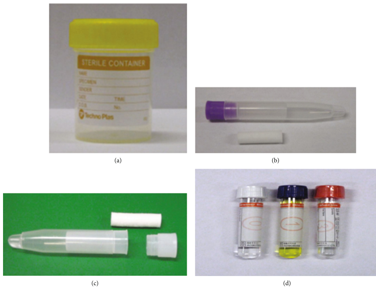
FIGURE 1: Commercially available saliva collection devices [44]. (a) Drool collected in a sterile specimen container. (b) SalivaBio Oral Swab (SOS) (Salimetrics, Carlsbad, California, the United States). (c) Salivette: cotton and synthetic swab (Sarstedt, Thermo Fisher Scientific, California, United States). (d) GBO Saliva Collection System (Greiner Bio-One, Kremsmünster, Austria).
