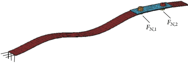
FIGURE 3: Finite-element model ( \approx 30000 DOFs and 632 nodes in contact) in typical bending deformation with the two screws that impose the external clamping force pairs F_{N,1} and F_{N,2} .
