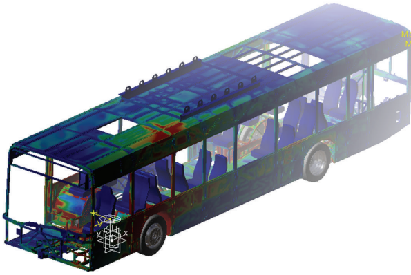
FIGURE 10: Hybrid urban bus model-stress Von Mises's measurement.
