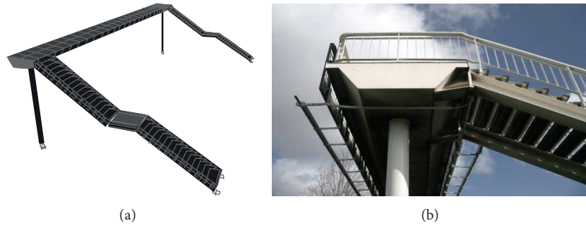
FIGURE 11: Steel box-girder structure under study: (a) analytical model; (b) view of column, deck, and stairway.
