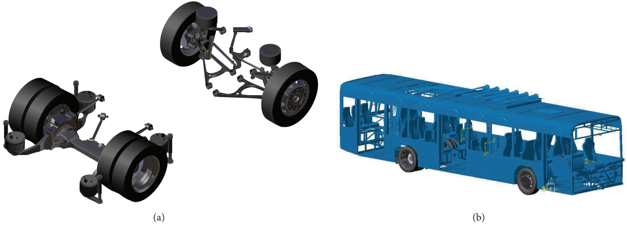
FIGURE 4: (a) Multibody bus suspension system; (b) rigid-flexible multibody bus model.
