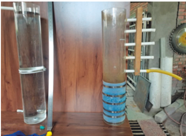
FIGURE 6: Non-Darcy flow permeability coefficient tester for compacted PFC-13 specimen.
