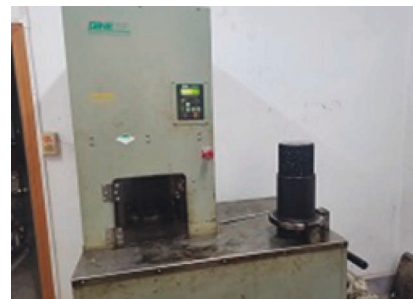
FIGURE 10: PFC-13 specimens prepared with a gyratory compactor.
