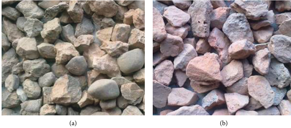
FIGURE 1: Macroscopic view of RA. (a) RCA, (b) RMA.
