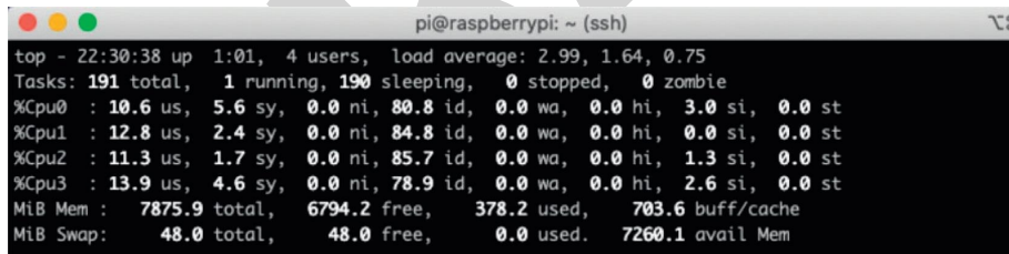
FIGURE 17: Average load under 1000 concurrent messages per second.
