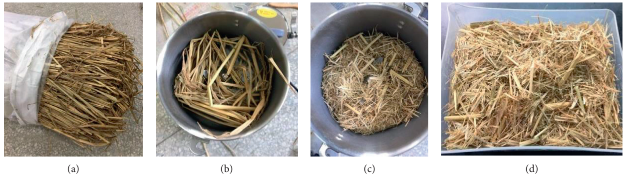
FIGURE 1: Pretreatment process of wheat straw. (a) Local wheat straw fibers. (b) Cleaned and dried fibers. (c) Milled fibers. (d) Fibers kept in a sealing bag.
