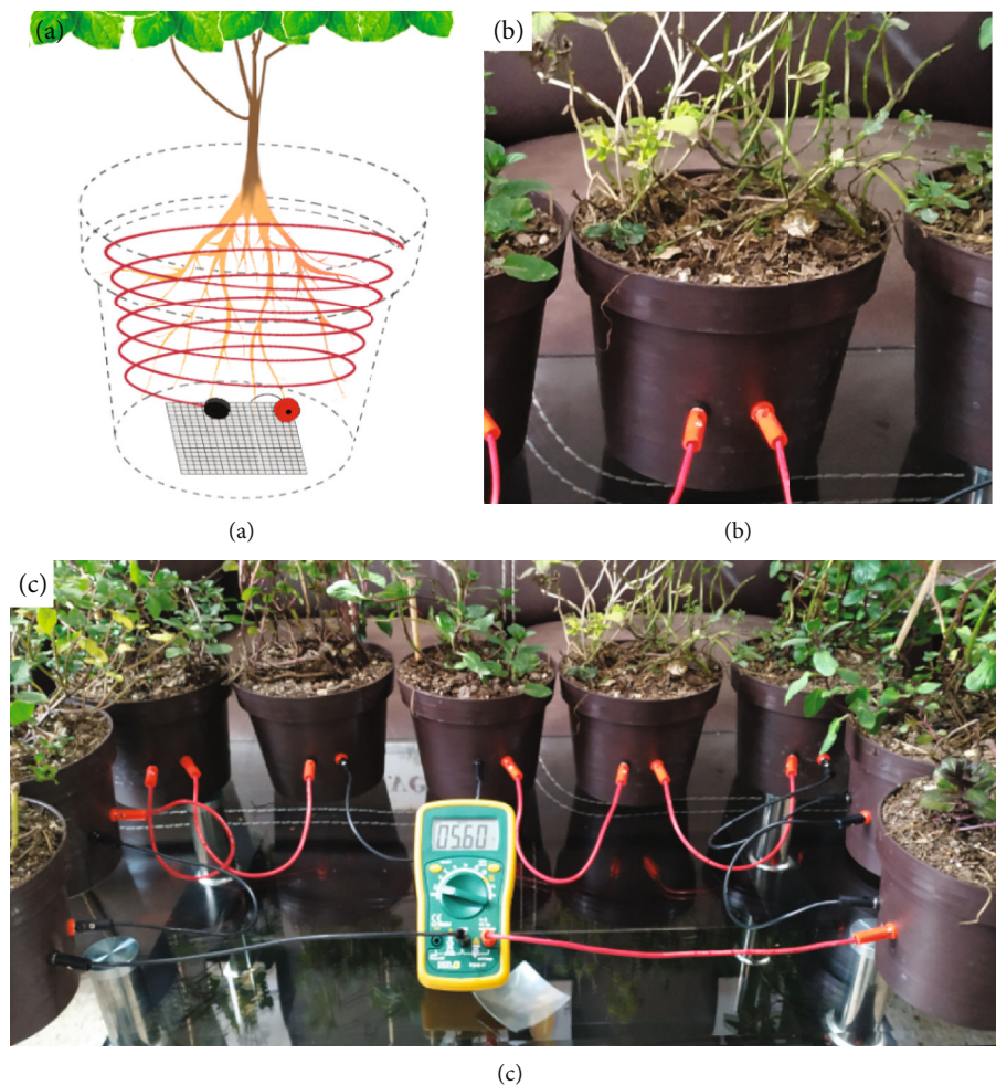
FIGURE 9: (a) Internal setup of the experiment inside the pot of the mint plant. (b) Electrodes of the mint plant. (c) A series of mint plants and the measured open-circuit voltage at the ends of the series.
