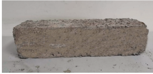
FIGURE 10: Cement-stabilized crushed stone molding test piece.
