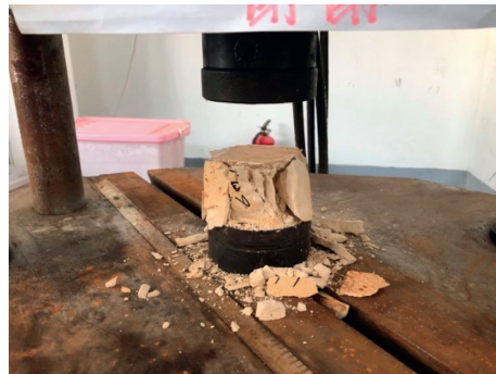
FIGURE 5: Compressive strength tests of the gypsum specimen.
