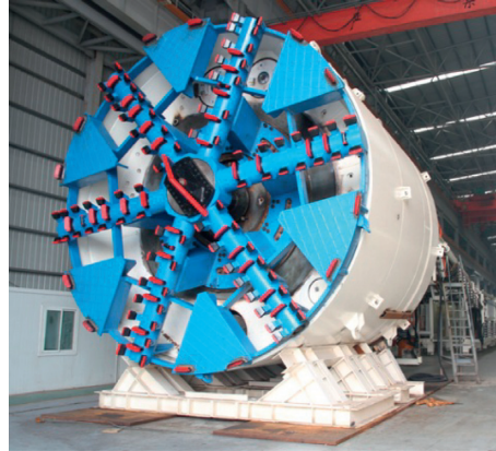
FIGURE 31: Picture of EPB shield.
