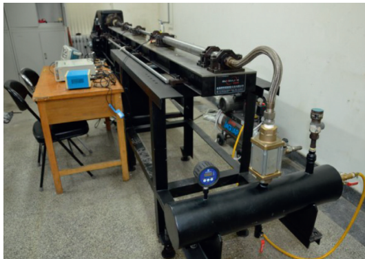
FIGURE 2: Physical drawing of the rotation-impact simulation system.
