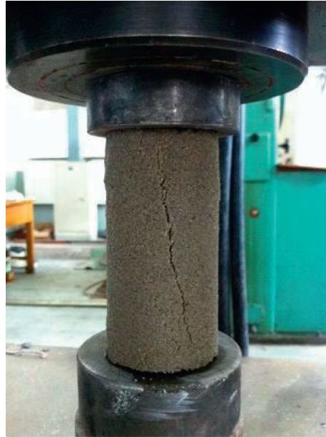
FIGURE 3: Failure of a saturated specimen.
