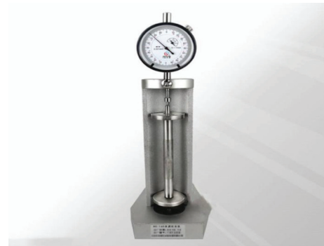
FIGURE 1: Comparator and dial indicators.
