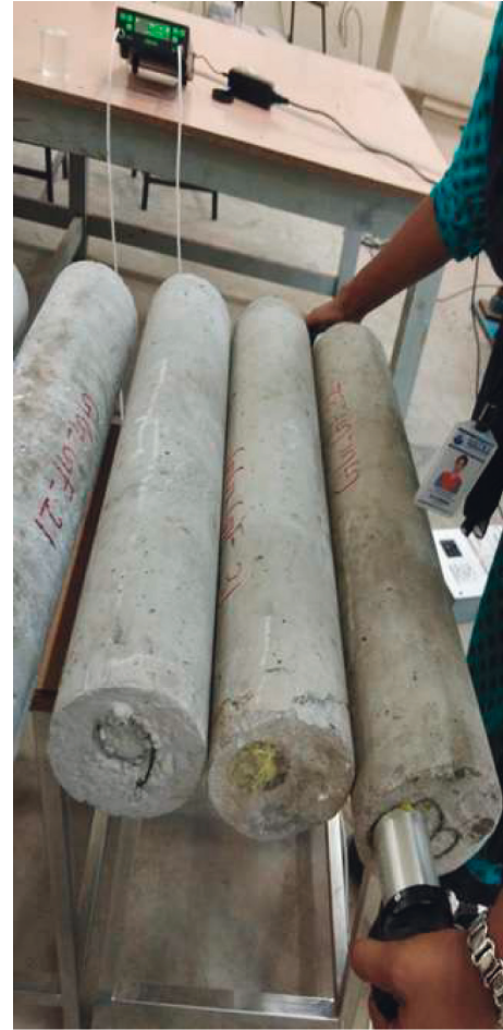
FIGURE 9: UPV test being conducted on column specimens.
