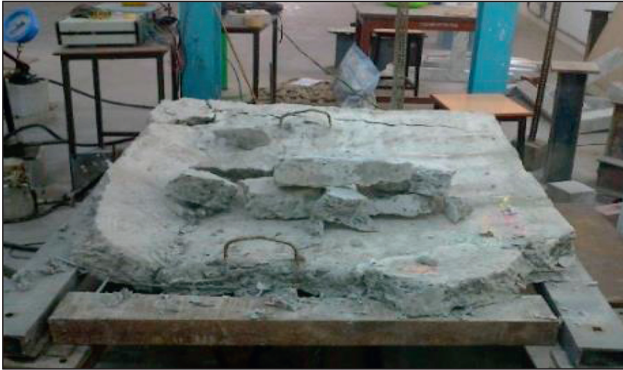
FIGURE 13: Final brittle collapse of glass fiber reinforced paper mass slab.
