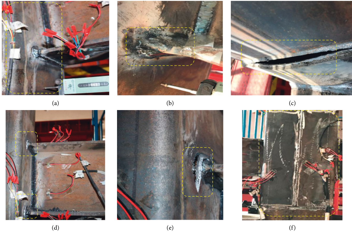
FIGURE 6: Failure modes of specimens. (a) Sleeve local buckling; (b) base metal tearing of the left; (c) weld cracking; (d) base metal tearing of upper; (e) sleeve tearing; (f) joint failure.
