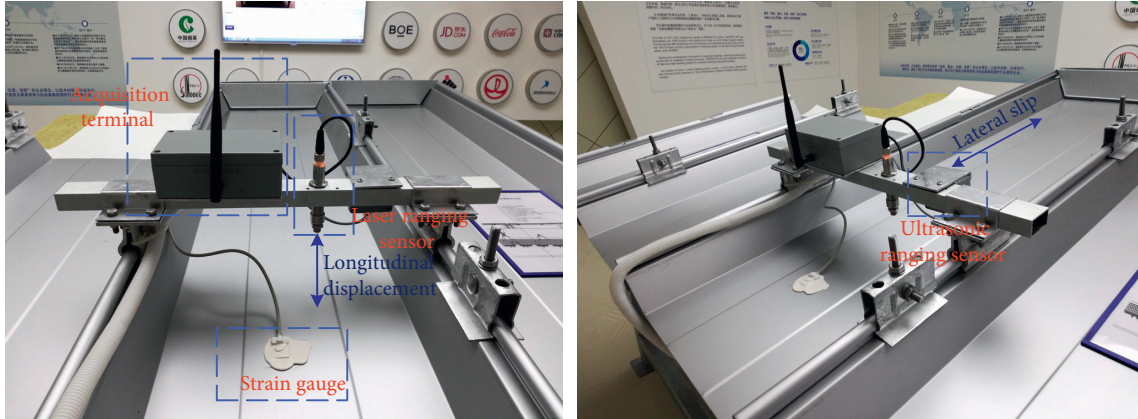
FIGURE 4: Terminal node sensor layout.
