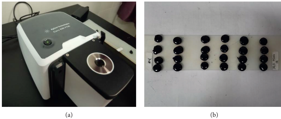
FIGURE 4: Infrared spectrum test of asphalt: (a) infrared spectrometer; (b) asphalt samples.
