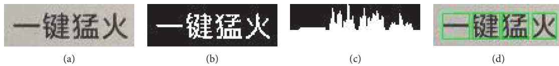
FIGURE 8: Projection-based character segmentation: (a) object region detected in the previous object localization step; (b) binary image of (a); (c) pixel distribution map obtained from the vertical projection of (b); (d) character segmentation obtained according to the peaks and valleys in the pixel distribution map in (c).
