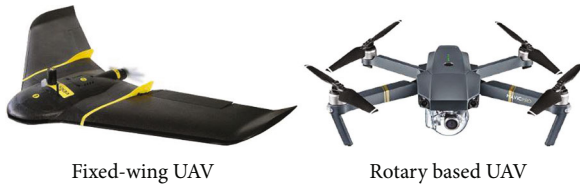
FIGURE 2: Two main types of UAVs.
