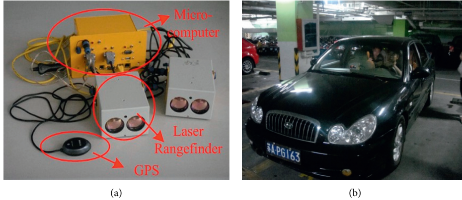
FIGURE 3: The device system and the instrumented vehicle. (a) The device system includes a laser rangefinder, a GPS device, and a microcomputer. (b) The instrumented vehicle is a Hyundai Sonata with an engine displacement of 2.0.
