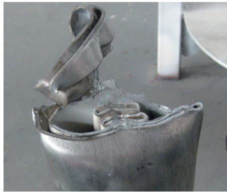
FIGURE 6: Fault surface of series cutting.
