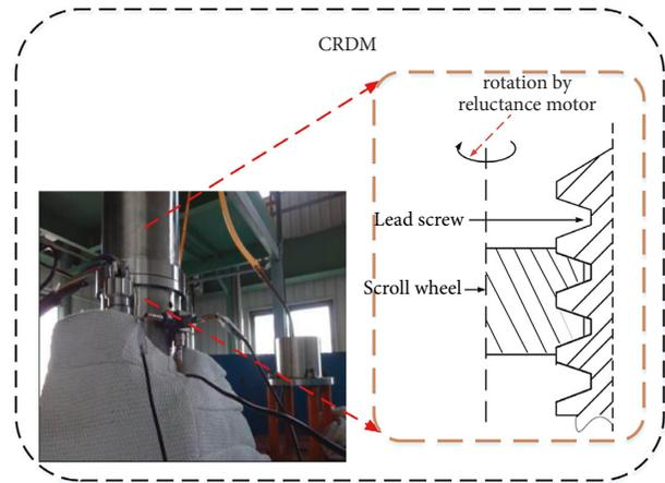
FIGURE 1: The sketch of the reluctance motor type CRDM.
