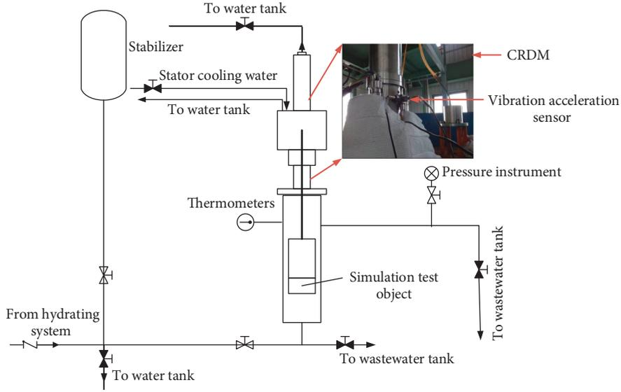
FIGURE 4: Schematic diagram of the CRDM full life test device.
