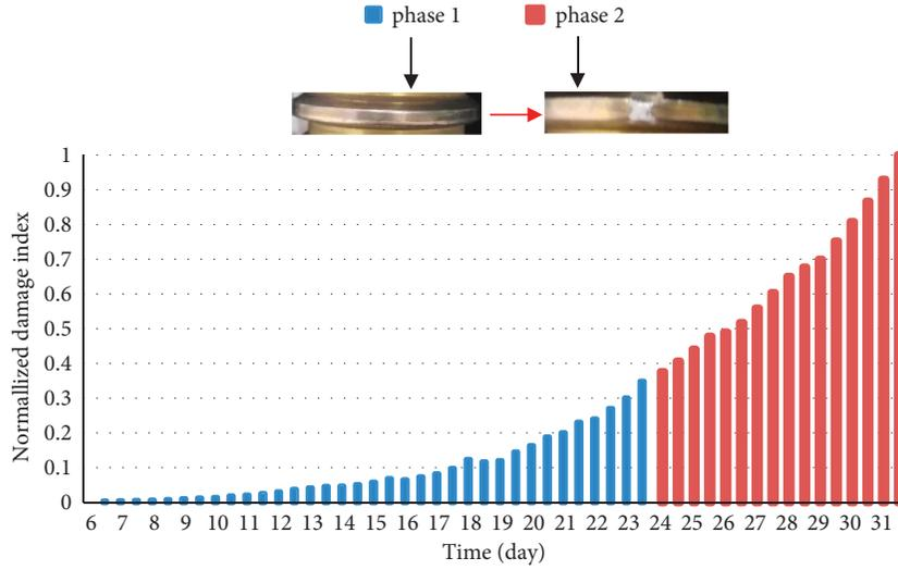
FIGURE 8: The segmented degradation process of the scroll wheel.
