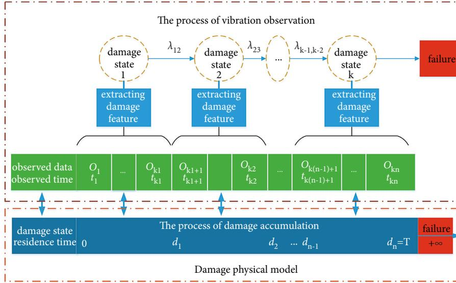
FIGURE 2: The relationship between the equipment observation process and damage process.
