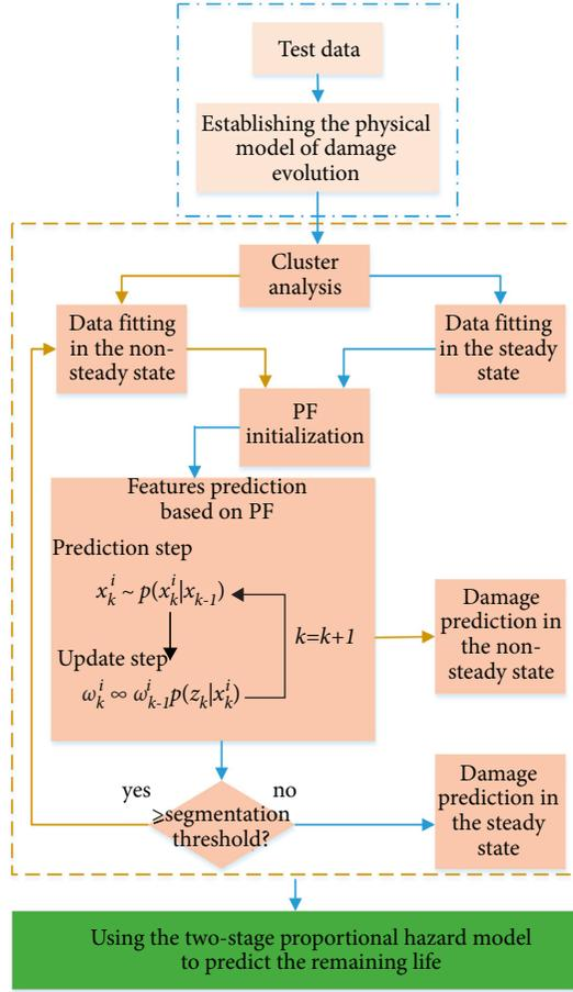
FIGURE 3: The framework to predict the remaining useful life of the scroll wheel.
