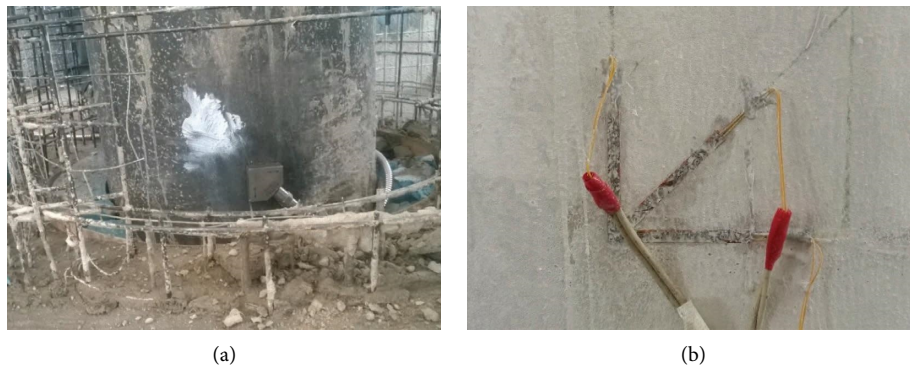
FIGURE 13: Sensor installation diagram. (a) Acceleration sensor of equipment outer wall; (b) strain gauges on wall.
