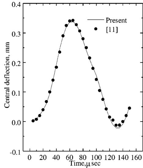
Fig. 6. Central deflection versus time for a  $0^\circ/90^\circ/0^\circ$  square clamped laminated plate with suddenly applied pulse loading ( $4 \times 4$  mesh).
