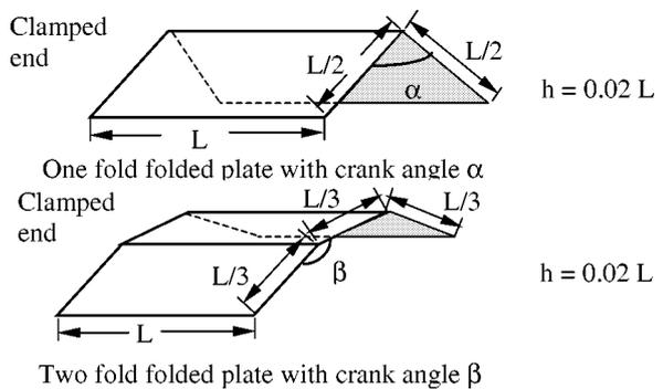
Fig. 3. Geometry of the folded plate used in examples 1, 2, 4, 5 and 6.
