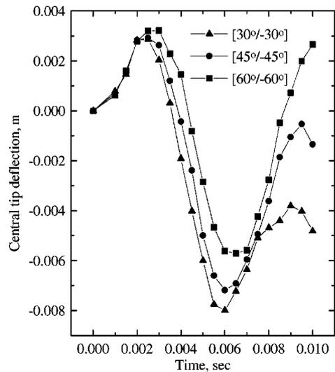
Fig. 7. Comparative central tip deflection versus time for 2-fold E-glass-Epoxy 2 layered folded plate with crank angle  $\beta = 120^\circ$  for various fibre angles (ref. Fig. 3) with  $L = 1.5$  m and suddenly applied step load  $q = 1.0 \times 10^5$  N/m<sup>2</sup>.
