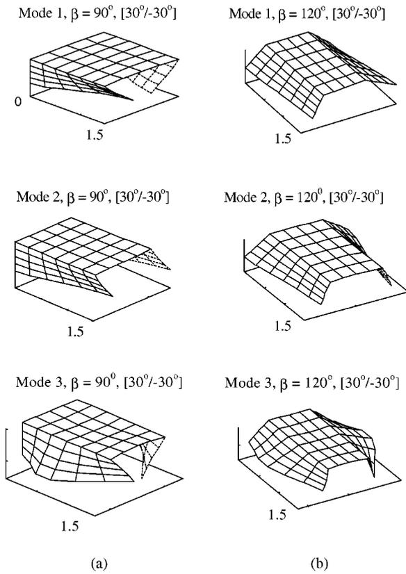
Fig. 5. First, second and third mode shapes of E-glass-Epoxy composite twofold folded plate with (a) crank angle  $\beta = 90^\circ$ , ply arrangement  $30^\circ/-30^\circ$ , and (b) crank angle  $\beta = 120^\circ$ , ply arrangement  $30^\circ/-30^\circ$ .
