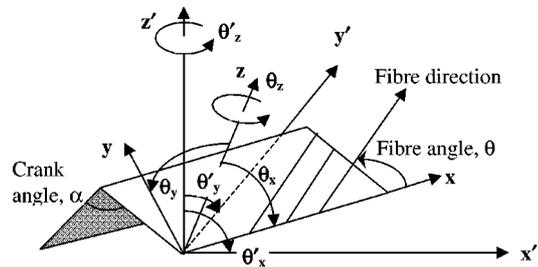
Fig. 2. Local (unprimed) and global (primed) axes system for a typical folded plate element. The least angle contained between positive  $x'$  and  $x$  axes is denoted as  $(x', x)$ .
