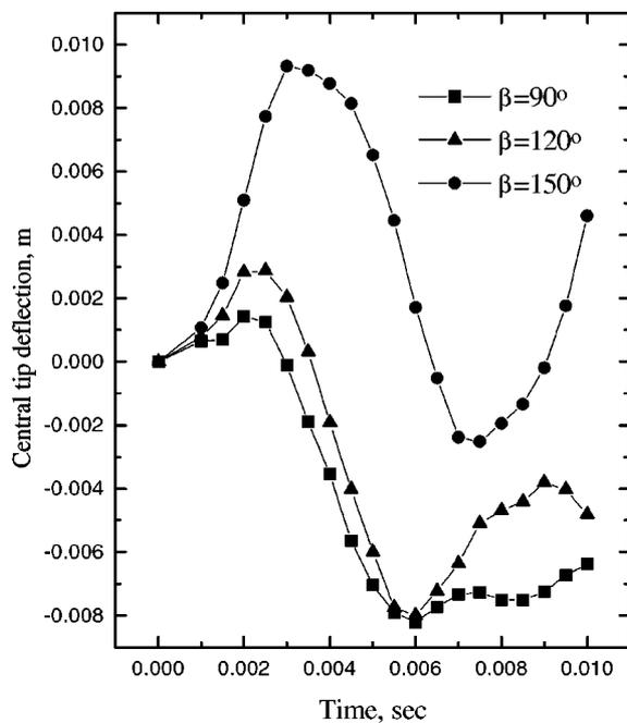
Fig. 9. Comparative study of central tip deflection for E-glass-Epoxy 2 fold laminated cantilever folded plates, with  $30^\circ/-30^\circ$  lamination,  $6 \times 3$  mesh.
