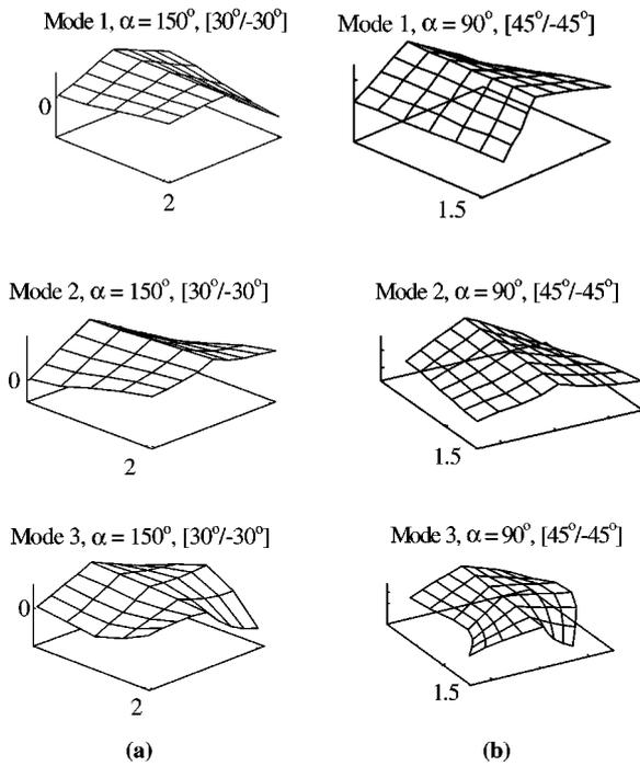
Fig. 4. First, second and third mode shapes of E-glass-Epoxy cantilever composite single fold folded plate with (a) crank angle  $\alpha = 150^\circ$ , ply arrangement  $30^\circ/-30^\circ$ , and (b) crank angle  $\alpha = 90^\circ$ , ply arrangement  $45^\circ/-45^\circ$ .
