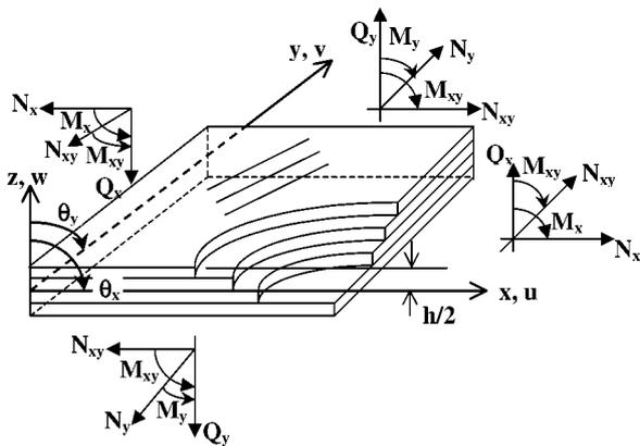
Fig. 1. The laminated composite plate with positive displacements, rotations and stress resultants.
