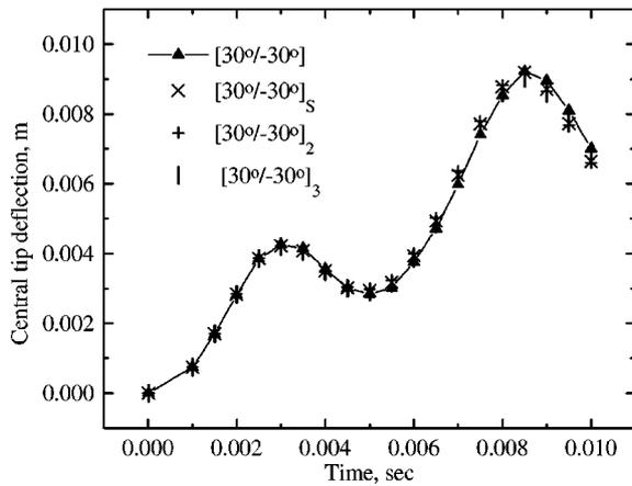
Fig. 8. Central tip deflection versus time for a cantilever single-folded plate with crank angle  $\alpha = 120^\circ$ , subjected to suddenly applied pulse loading ( $4 \times 3$  mesh).
