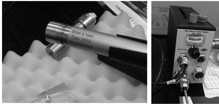
Fig. 67. Brüel & Kjær type 2669 Microphone and power supply unit.
