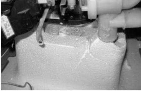
FIGURE 7: The broken bottom cushion pad after the shock test at a 400 mm drop height.
