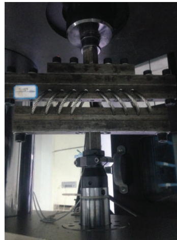
(b) The actual setup of an isolator under tension-compression loading
