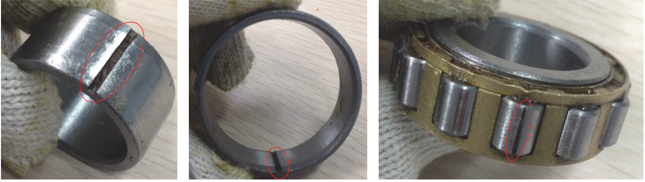
FIGURE 4: Faults of inner ring, outer ring, and roller element.
