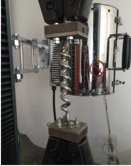
FIGURE 3: Large-scale SMA helical spring.
