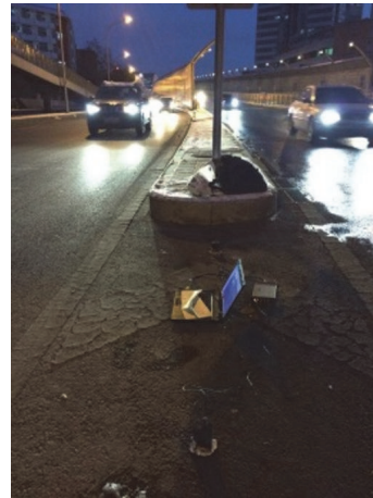
FIGURE 18: Field tested acceleration along a road.
