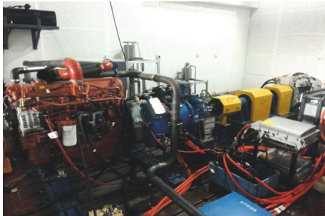
FIGURE 9: Bench test-bed for new hybrid electric system.
