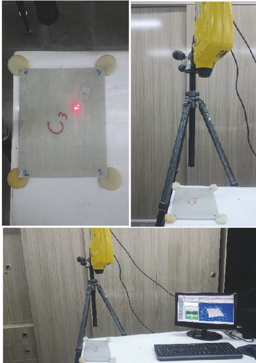
FIGURE 3: Modal test for thin glass/epoxy plates (F-F-F-F).
