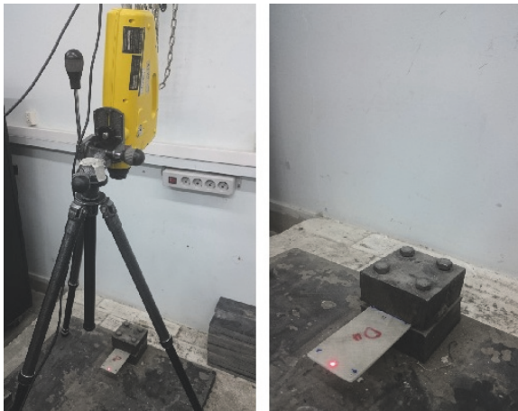
FIGURE 4: Modal test for thick glass/epoxy plates (C-F-F-F).
