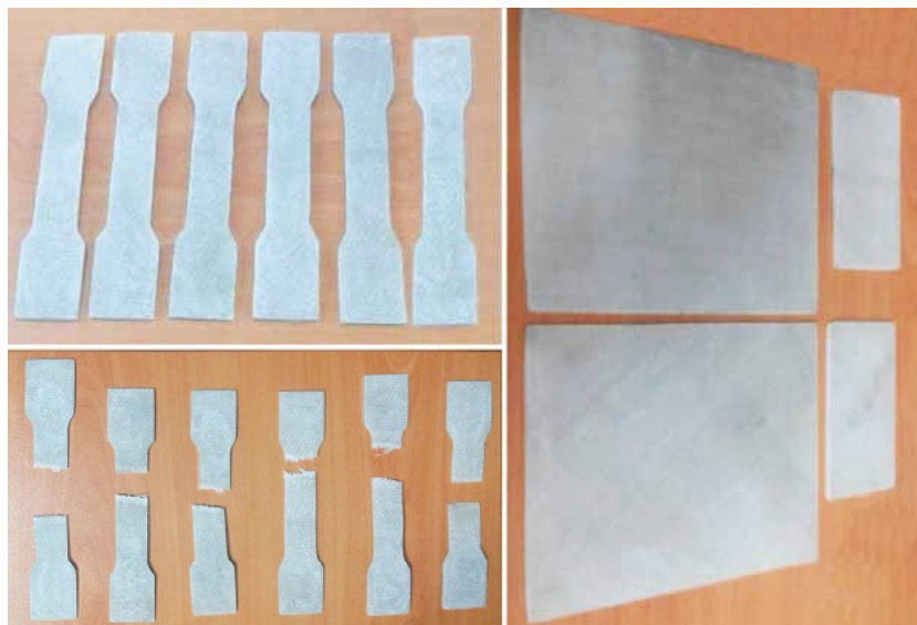
FIGURE 2: Glass/epoxy specimens for modal and tensile tests.
