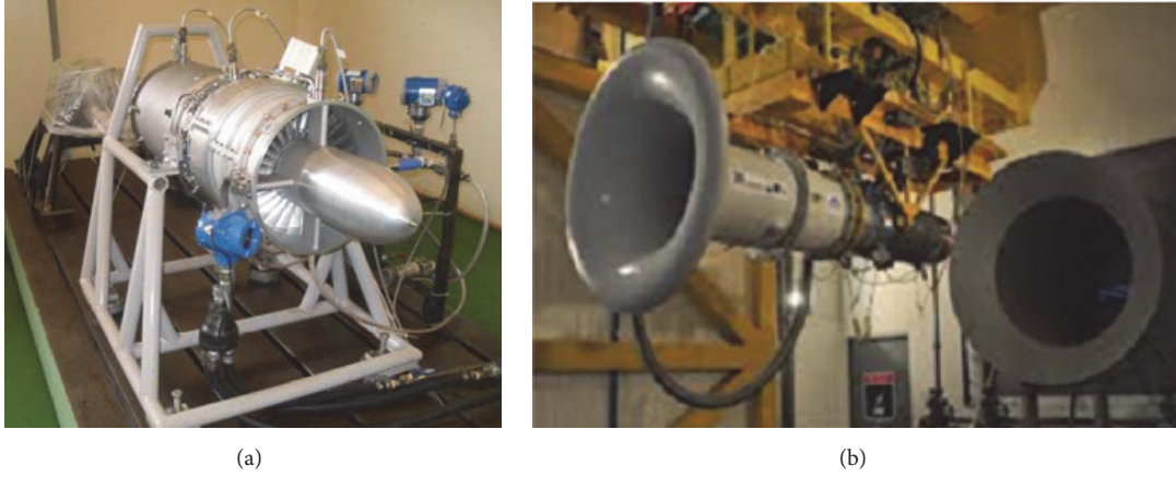
FIGURE 1: Manufactured single spool gas turbine developed in this study: (a) apparatus for demonstrative purposes and preliminary tests and (b) test rig for full test protocol.
