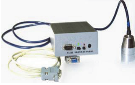
FIGURE 4: TOPBOX-508 vibration signal recording apparatus.
