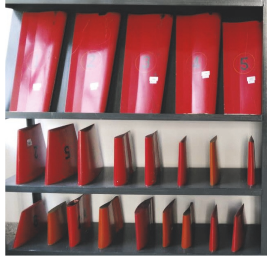
FIGURE 2: Experimental fins used in water tank experiment.
