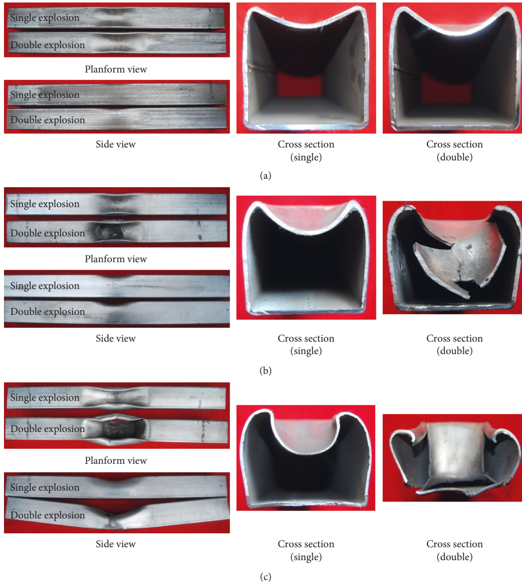
FIGURE 8: The deformation and damage comparison of square tubes subjected to single and double explosions. (a) a = 4.0 mm, R = 20 cm. (b) a = 3.5 mm, R = 14 cm. (c) a = 3.0 mm, R = 12 cm.
