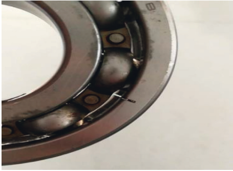
FIGURE 7: The fault diameter 0.5 mm outer race defect of the test rolling bearing.
