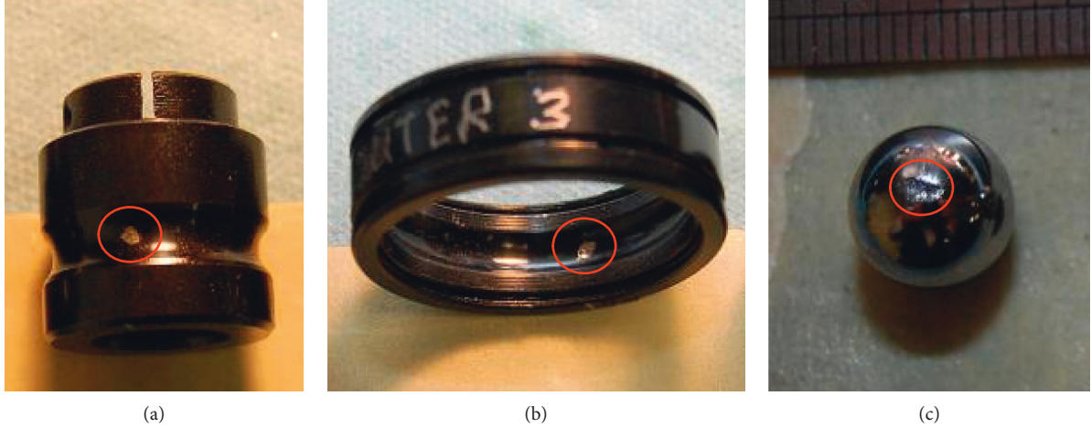
FIGURE 4: Pictures of the bearing faults: (a) IF; (b) OF; (c) BF.
