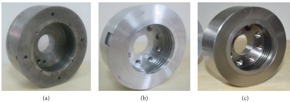
FIGURE 12: Assembled balance terminal. (a) Steel-45#. (b) Aluminum alloy-7A04. (c) Titanium alloy-TC4.
