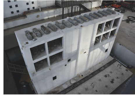
FIGURE 3: Counterweighting the test model.
