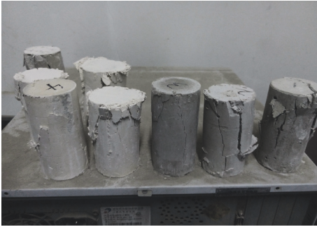
FIGURE 2: Typical compressive fracture failure modes.
