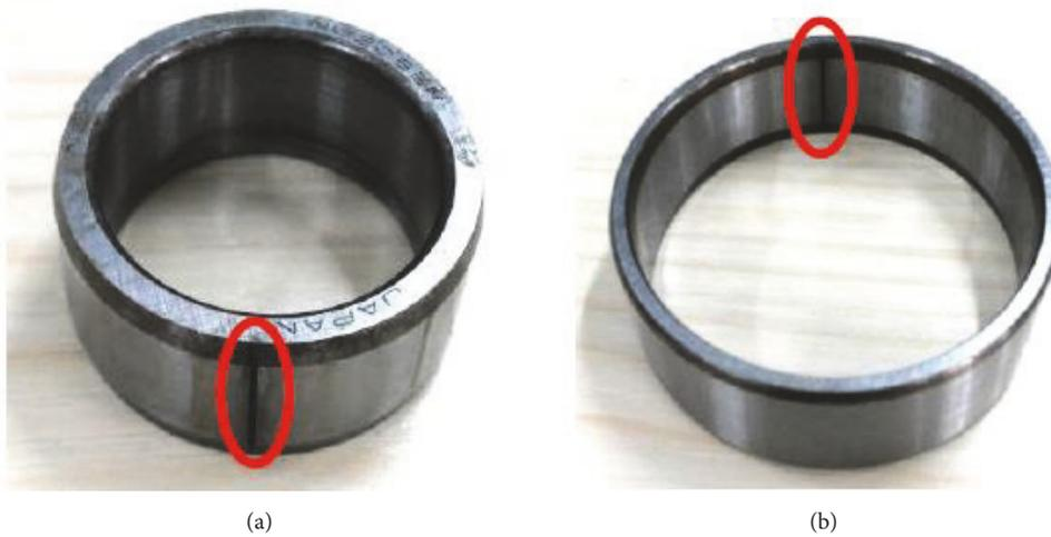
FIGURE 6: Fault bearings. (a) Outer-race fault; (b) inner-race fault.
