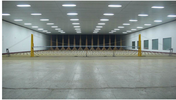
FIGURE 9: Test model of the suspension bridge.
